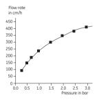
Fig 3. Pressure/flow rate curves for SP Sepharose High Performance. BPG 200/500 column, bed height 10 cm, distilled water.
