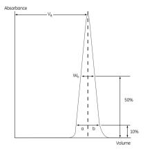
Fig 5. A typical test chromatogram showing the parameters used for HETP and  $A_{\rm s}$  calculations.
