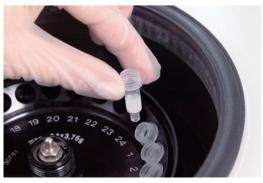
Fig 3. GST SpinTrap columns are designed for efficient, small-scale purification of GST-tagged proteins using a microcentrifuge.
