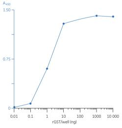
**Fig 10.** Sensitive detection of recombinant GST using the GST 96-Well Detection Module. The indicated amounts of rGST protein were applied directly to the wells of a GST 96-Well Capture Plate. After binding and washing, the wells were treated with a HRP/Anti-GST Conjugate, and detection was performed adding 3, 3', 5, 5'-tetramethylbenzidine (TMB) substrate ( $A_{450}$ ).
